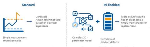
The health status of the slurry pumps is traditionally monitored via a single measurement, i.e. an amperage spike. If a spike occurs the operator acts based on experience, an unreliable process that leads to pump failures and unplanned line downtime.
